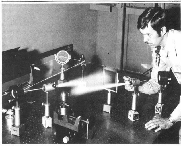
LABORATORY ARRANGEMENT for obtaining holograms. Dan Tichenor focuses beam on the target, the spherical vessel left of center.
